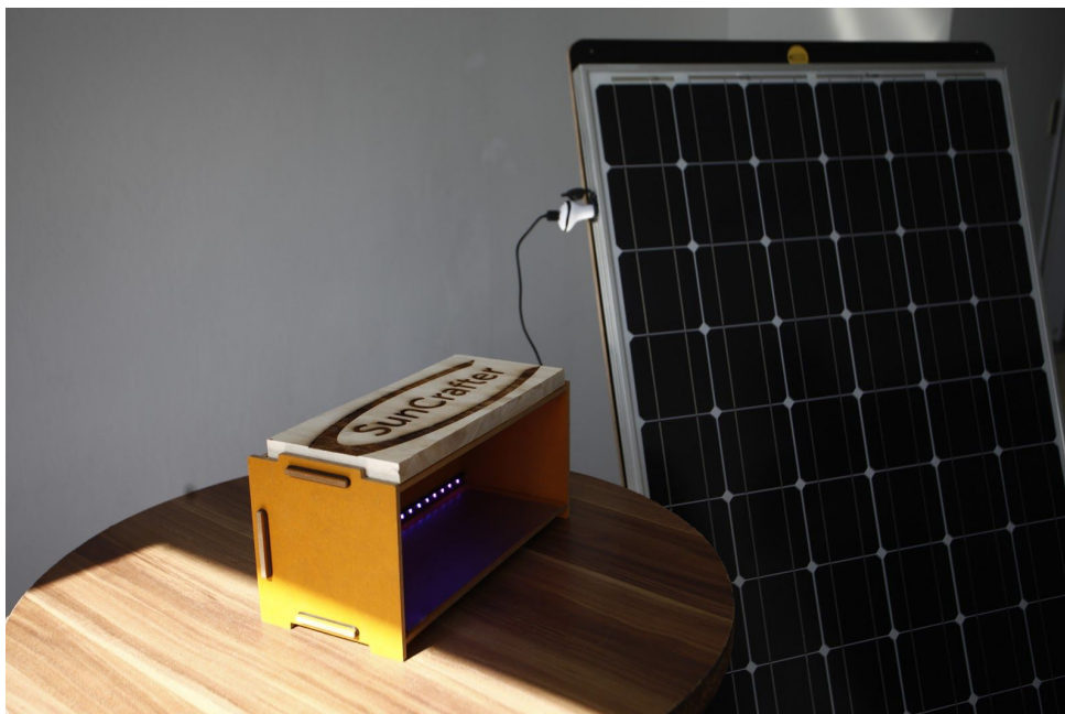
(UVC disinfection hub, powered by off-grid solar system EasyPanel. © 2020 by SunCrafter)
